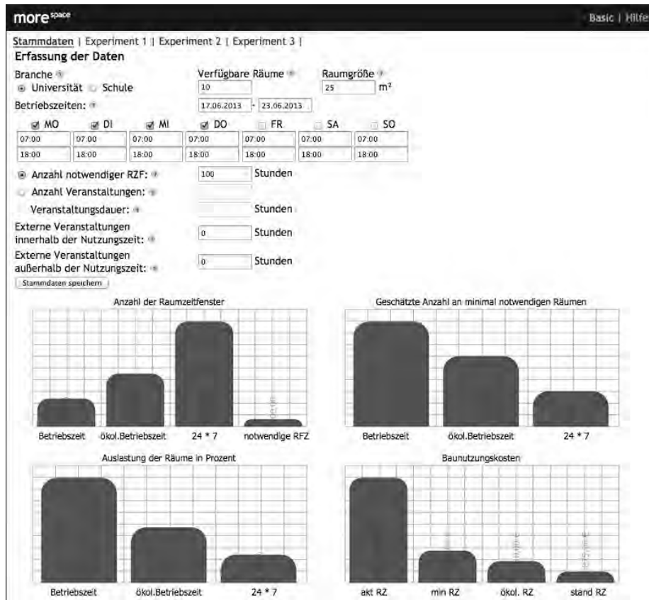
Figure 4.19: Master tab of static analysis tool (STAN, version “Basic”), intended to facilitate system understanding and awareness raising for impact of space utilization.
