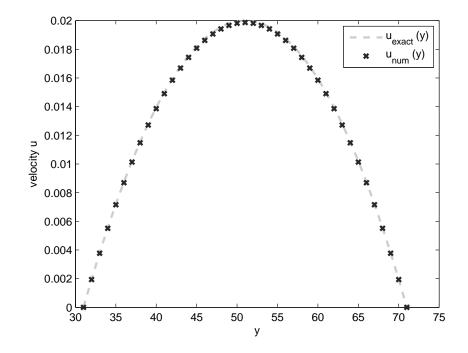
Figure 5.18: Comparison between computed velocity profile (blue) and analytical solution of Poiseuille (green) with density difference  $\Delta \rho = 0.02$  between inlet and outlet (inlet/outlet BC)
