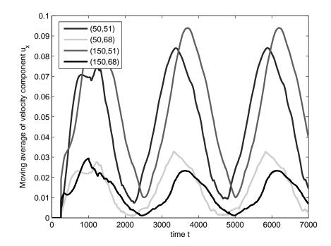
Figure 5.23: Moving average over 250 time steps of the velocity component  $u_x$  at different lattice nodes (blue and red for a node with central y-coordinate, green and black for a node with y-coordinate near the upper wall)
