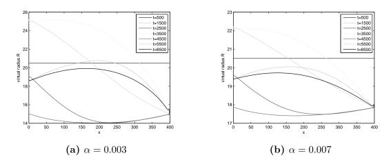
Figure 5.35: Virtual radius R at every position x for different points in time, gained from simulations with different  $\alpha$ . Expansion and contraction are allowed only after 1000 time steps when the flow is fully developed. Hence, at t = 500, the channel keeps its initial state (straight).
