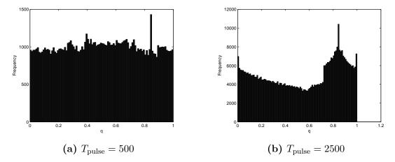
Figure 5.41: Histograms for the parameter q of the continuous bounce-back condition at the lower boundary over one pulse period, gained from simulations with different  $T_{\text{pulse}}$ . In each case, the prominent peak (around 0.85) is due to the boundary condition at the outlet which bounds the outlet section because of the prescribed constant pressure (and as a consequence constant q).
