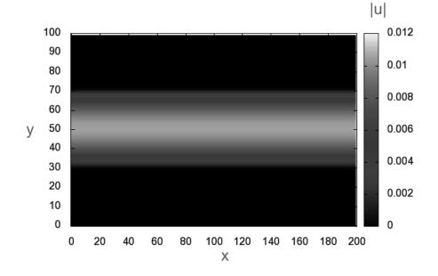
channel. The maximum velocity of 0.01 (compare with Fig. 5.4) is correctly reached in the center of the channel.
