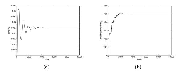
**Figure 5.20:** Time history of the density  $\rho$  (a) and the velocity component  $u_x$  (b) at the center node of the channel
