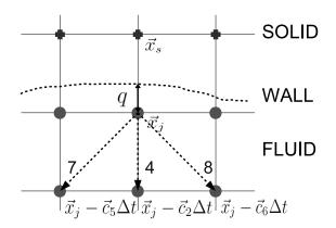
Figure 3.8: Continuous bounce-back boundary condition for a virtual wall located at distance q from the last fluid node  $x_j$ . Gray crosses indicate solid nodes, red filled circles denote fluid nodes. The lattice spacing  $\Delta x$  is set to one. Dashed blue arrows represent directions i of unknown populations  $f_i$  which are determined using the linear interpolation in Eqs. 3.29 or 3.30.
