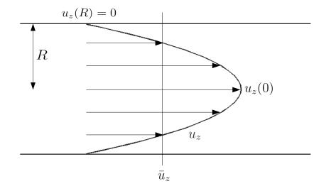
Figure 2.2: The parabolic velocity profile  $(u_z)$  of a fully developed steady Poiseuille flow. The average velocity  $\bar{u}_z$  is one half of the maximum velocity. At the wall, the velocity is zero (no-slip condition).
