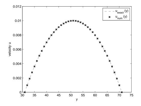
**Figure 5.4:** Velocity: Comparison between analytical solution of Poiseuille (green) and numerical result (blue) (periodic BC)
