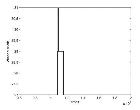
Figure 5.45: Width of the channel at the outlet as a function of time as a response to the single pulse given by Eq. 5.10. Coupled LBM/WK used with  $C = 10^4$  and R = 0.5.
