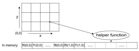
**Figure 5.3:** Example of memory allocation for the distribution functions  $f_i(x, y)$ . The helper function translates x, y and i from a matrix form to the position in the linear array.
