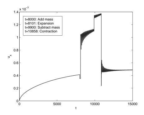
Figure 5.16: Velocity component  $u_x$  at fluid node next to the wall as a function of time, lower viscosity ( $\nu = 1/30$ ), compare with Fig. 5.8
