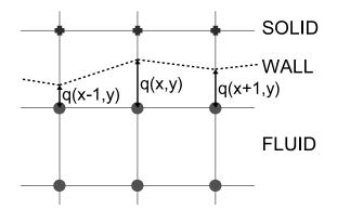
Figure 4.5: Continuous bounce-back boundary condition for a virtual wall located at distance q from the last fluid node. To every fluid node next the the wall a different q is assigned. Gray crosses indicate solid nodes; red filled circles denote fluid nodes. The lattice spacing  $\Delta x$  is set to one.
