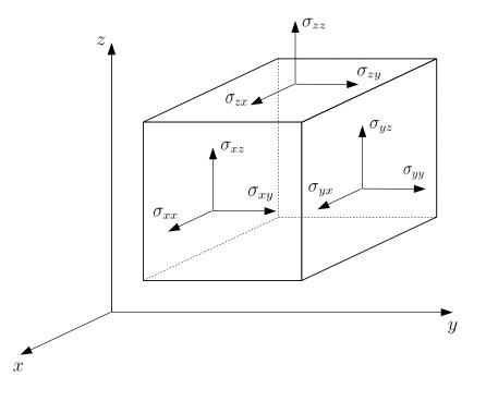
Figure 2.5: Components of the stress tensor on an infinitesimal cubic element in the Cartesian coordinate system
