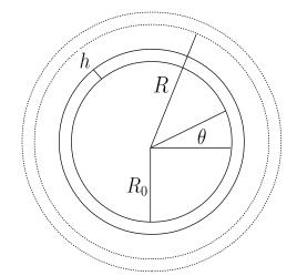
Figure 2.6: Transversal section of a tube of thickness h
