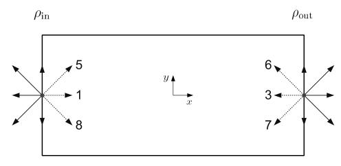
Figure 3.9: Inlet/outlet boundary conditions. Dashed arrows indicate unknown populations; full arrows denote known particles.
