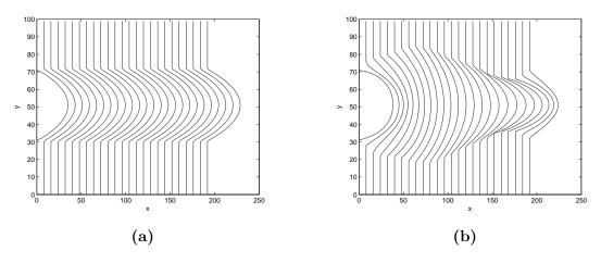
Figure 5.19: Velocity profiles of fully developed flow along x in a rigid straight channel (a) and a rigid channel with curved walls (b)
