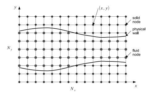
Figure 5.1: Sketch of lattice with embedded vessel
