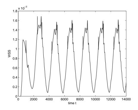
Figure 6.3: Wall shear stress at the upper wall at the beginning of the stented segment as a function of time ( $\alpha_0 = 0.07, \sigma = 50$ )
