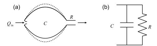
Figure 5.42: The Windkessel model (a) and the equivalent representation as electric circuit (b). Q<sub>in</sub> is the flow into the Windkessel, C denotes the compliance/capacitance and R represents the resistance.
