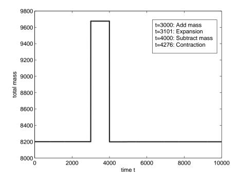
Figure 5.6: Total mass as a function of time. In order to better distinguish between the single steps (1. to 5., see text), the algorithm waits for at least 100 time steps and for fully developed flow before performing the next step.
