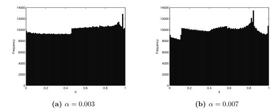
Figure 5.36: Histograms for the parameter q of the continuous bounce-back condition at the lower boundary over one pulse period, gained from simulations with different  $\alpha$ . In each case, the prominent peak is due to the boundary condition at the outlet which bounds the outlet section because of the prescribed constant pressure, see Eq. 5.4 (and as a consequence constant q).
