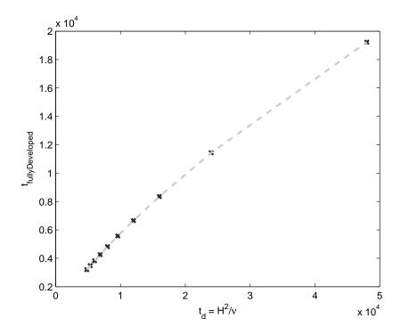
Figure 5.13: Time at which flow is fully developed as a function of the diffusive time  $t_d$  ( $\nu$  variating)
