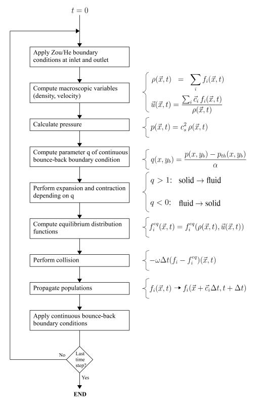
Figure 5.2: Flow chart of the implemented lattice Boltzmann algorithm
