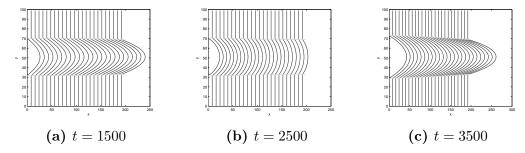
Figure 5.29: Profiles of the velocity component  $u_x$  along the channel at three instants in the case of oscillating inlet pressure. The scale of these figures do not allow a precise resolution, but the channel in case (b) is slightly more expanded than in case (a), and the channel in case (c) is more expanded than in case (a) and (b). The wall displacement of just one or two lattice units is not clearly visible in the figures.
