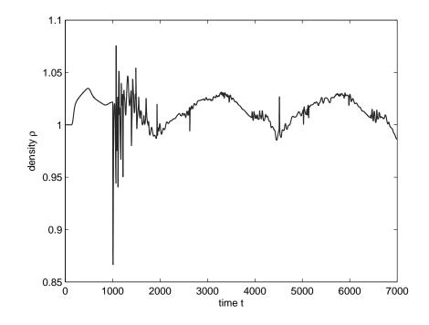
Figure 5.21: Density  $\rho$  as a function of time at a node near the wall (bounce-back on the link, see Section 3.3.2)
