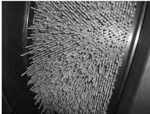
**Figure 2:** Pellets leaving the press (DVT 2017).
