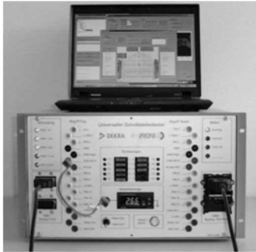
Fig. 2.1: Test environment with main user interface (univ. IT / univ. SST)
