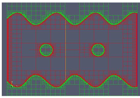
Figure 8: Driftratchet in 2D using Peano trees (a space-tree based upon tri-partitioning)
