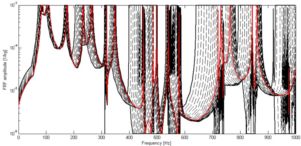
**Figure 5:** Frequency response of the plate, scenario 2.
