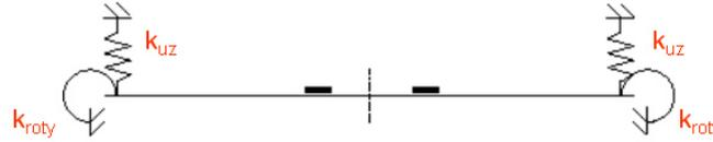
**Figure 2:** Side view of the plate: linear springs in  $z$ -direction/about  $y$ -axis with spring constants  $k_{uz}$  and  $k_{roty}$  simulate support uncertainties.
