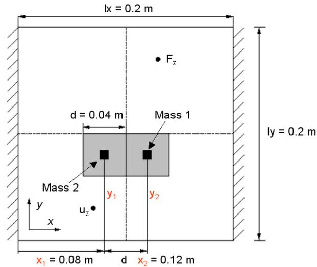
**Figure 1:** Top view of the plate with the range of uncertainty in the positioning of the two masses (grey), clamped on two sides.
