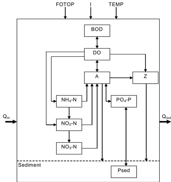
**Figure 1:** Conceptual model of the eutrophication simulator
