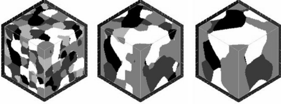
Figure 1: Simulation of the coarsening process of a polycrystalline grain structure at three subsequent times in 3D.
